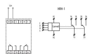
Terminals description: A1, A2 - supply voltage C - wire for both probes D - wire of bottom probe E2 H - wire of upper probe E1 S - earth terminal for possible screening of cable 15-16-18 output contact relay 1 25-26-28 output contact relay 2
