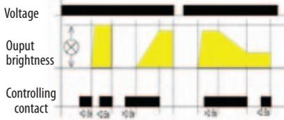
KA short press ( $<0.5s$ ) turns a light on, another short press turns it off. A longer press ( $>0.5s$ ) causes a gradual regulation of light intensity min-max-min round until the button is released. After releasing a set intensity is kept in memory, further short presses turn the light on/off keeping the set intensity. The intensity can be changed by further long press. After de-energising the relay remembers the set value.
